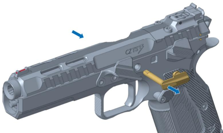
7. Push the slide assembly with the barrel and recoil assembly forward.
